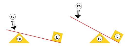
The closer the fulcrum (FU) is to the load to be lifted (L), the lower the force required (FO) will be needed to lift this load.
