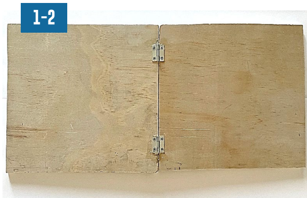
Plywood (3/8 inch) 2 surfaces of 23 x 30 cm 2 narrow hinges 2,5 x 2,5 cm
